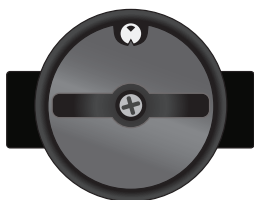
Fig D. To set bypass for green/blue scale mode, turn bypass wheel to show 1 segment in small circular window
