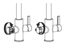
Run the boiling water side (the water will be cold at this point as the unit isn't plugged in). Press the button down and turn the handle to the boiling side. It may take a little while for the water to come through the system. Once water is running, close tap off and check for leaks.
