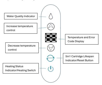
To set your desired water temperature (37°C to 98°C), use the up and down arrows on the unit until your temperature shows on the screen. Press the up and down arrows to increase/decrease by 1°C at a time. Or hold the buttons to change the temperature quickly. Once set, the unit will display the current temperature in the unit.
