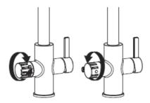
Run the boiling water side (the water will be cold at this point as the unit isn't plugged in). Slide the 'pik' out and turn the handle to the boiling side. It may take a little while for the water to come through the system. Once running, turn the tap off and check for leaks.
