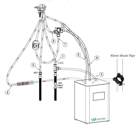
Finally, tidy up all the hoses, so they don't get tangled up. Please leave enough space for the pull-down hose with counterweight to move up and down without interference to ensure the pull-down function and return works. The three-way connector (M) can be attached to the wall. Screw clip (N) into the desired location and clip the three-way connector (M) to the clip.
